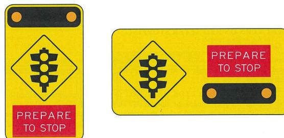
Examples of supplementing signs with alternating flashing yellow lights shown in black area
