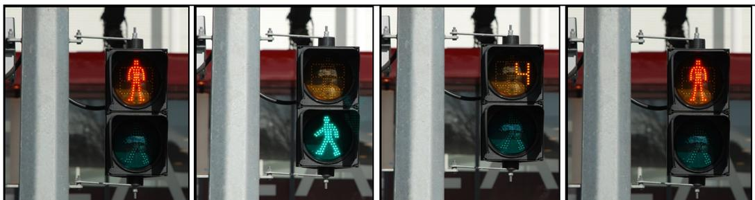
Figure 5.1 Pedestrian Countdown Timer Displays
