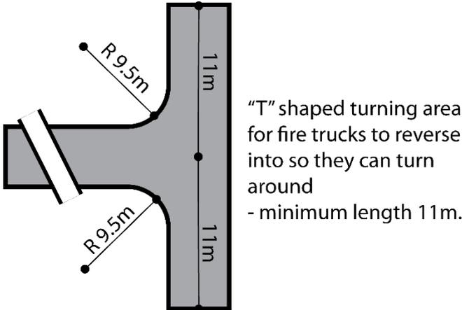
"T" shaped turning area for fire trucks to reverse into so they can turn around - minimum length 11m.
