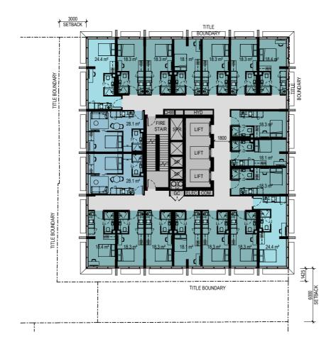
CLEANERS CUPBOARD COM COMMUNICATIONS RISER CHW CHILLED / HOT WATER RISER ELEC ELECTRICAL RISER GC GARBAGE CHUTES
