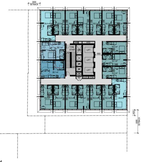
CLEANERS CUPBOARD COM COMMUNICATIONS RISER CHW CHILLED / HOT WATER RISER ELEC ELECTRICAL RISER
