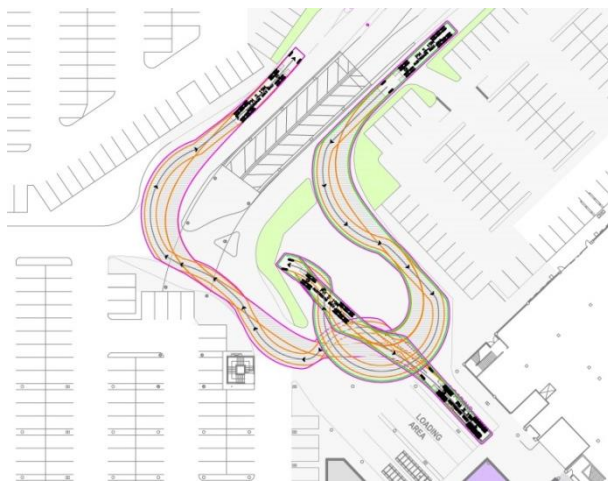
Figure 26: Swept Path of a commercial vehicle entering and exit the loading area in a forward direction
