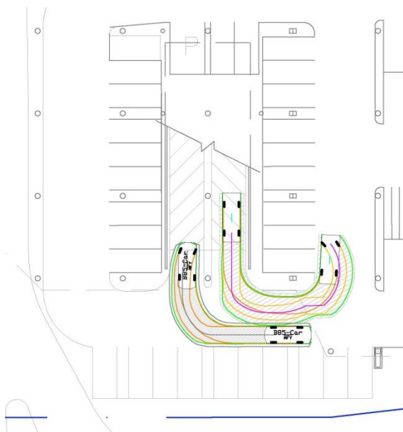
Figure 13: Connection of ramp to internal aisle creating minimal impact on traffic flow.
