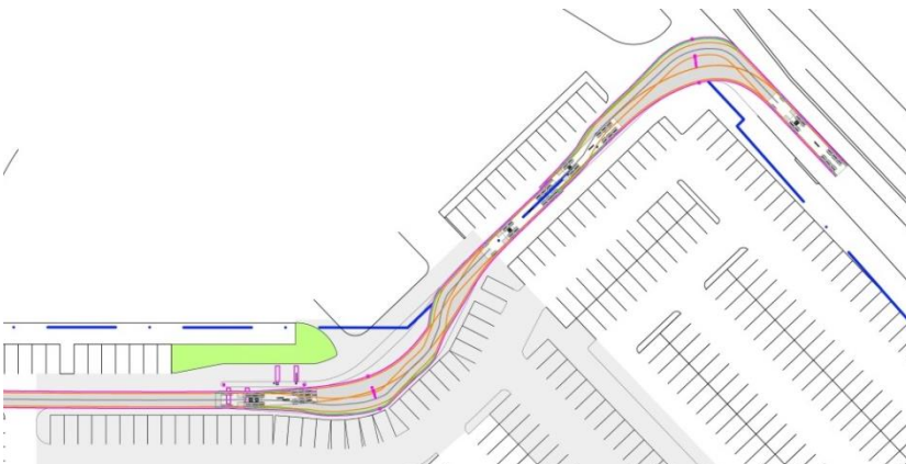
Figure 14: Swept path of semi-trailer entry movements at Access 12
