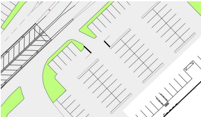
Figure 13: Separate internal connection facilitating egress movements to Diagonal Road
