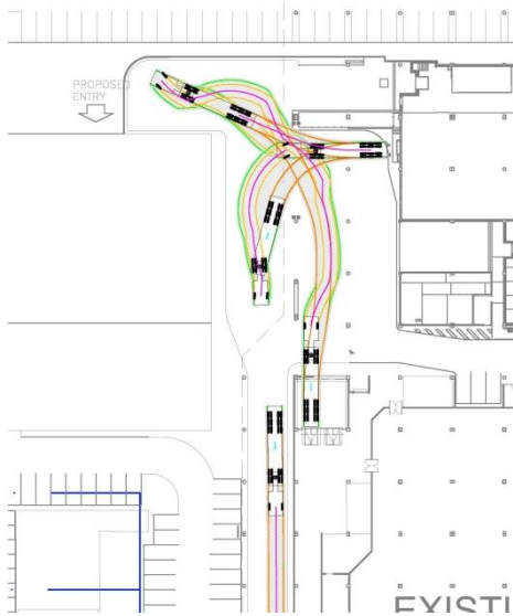
Figure 29: Swept path of turning semi-trailer turning to exit site.
