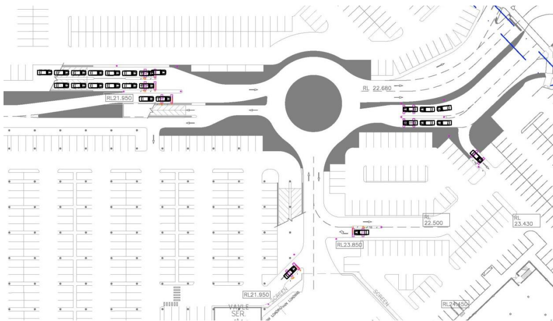
Figure 47: Forecast queues at the entry and exit gates adjacent the Diagonal Road signal.
