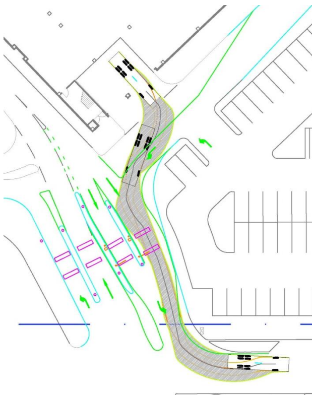
Figure 30: Access control equipment accommodating the existing egress movements
