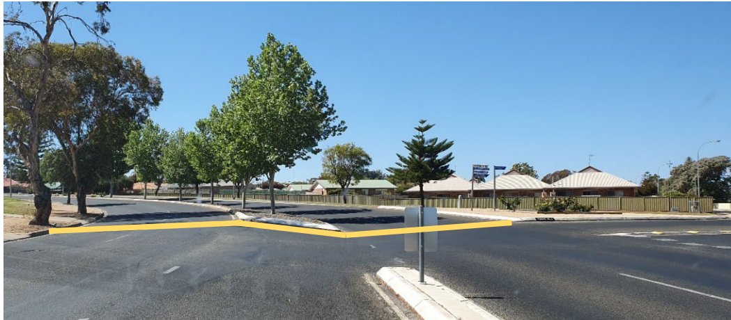
Figure 4 – The separately cambered ‘saw tooth’ carriageways (emphasised in yellow) of Kay Avenue at its intersection with Fernwick Road
