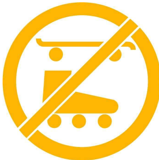
Figure 5.3 - 'All Skaters Prohibited' Pavement Marking
