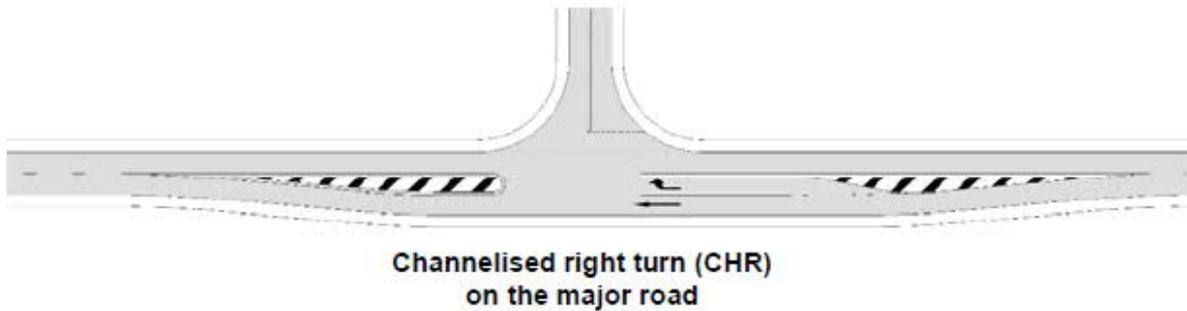
Figure 33: Example of a channelised right turn (CHR) treatment from major road (Source: Austroads)
