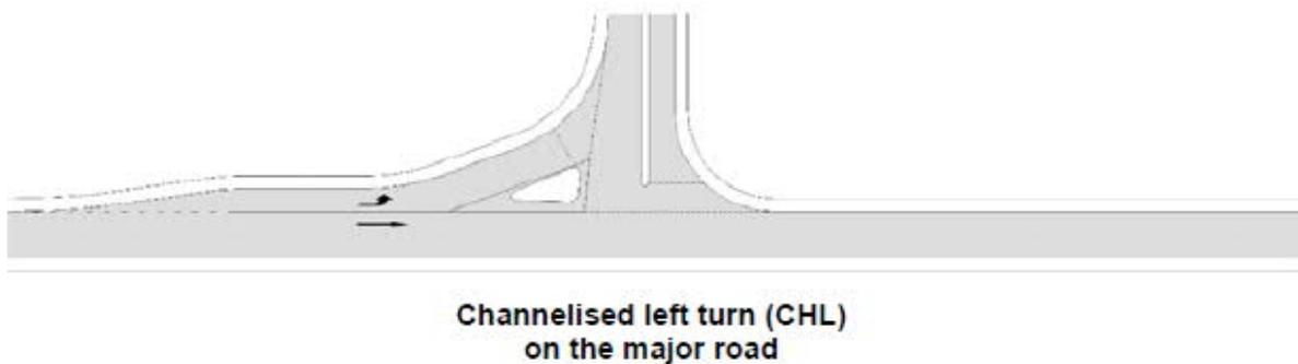
Figure 34: Example of a channelised left turn (CHL) treatment from major road (Source: Austroads)
