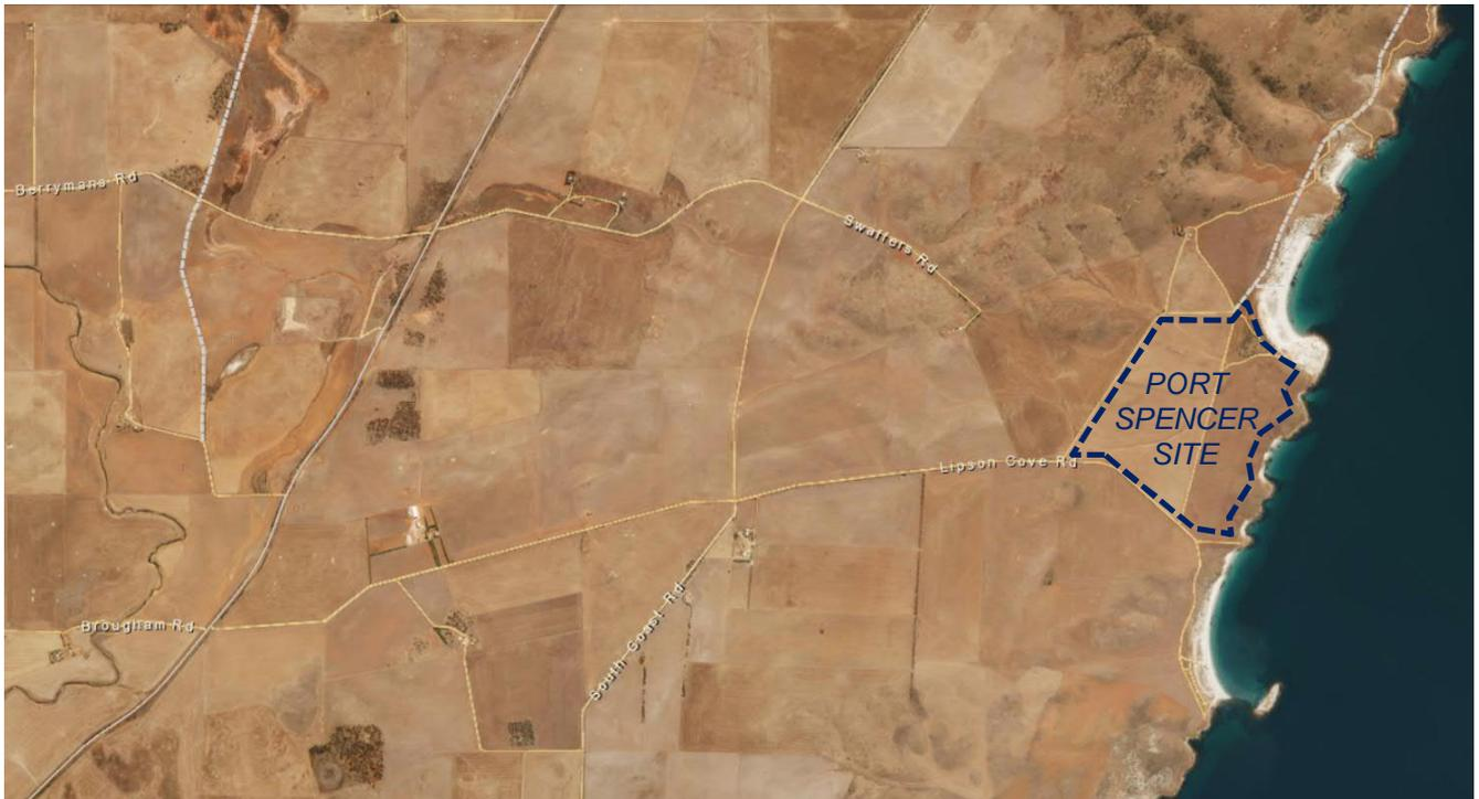
Figure 5: Sealed (solid grey line), unsealed (solid yellow line) and unformed roads (dashed grey line) in vicinity of the proposed site (dark blue outline) (Source: Location SA Viewer)
