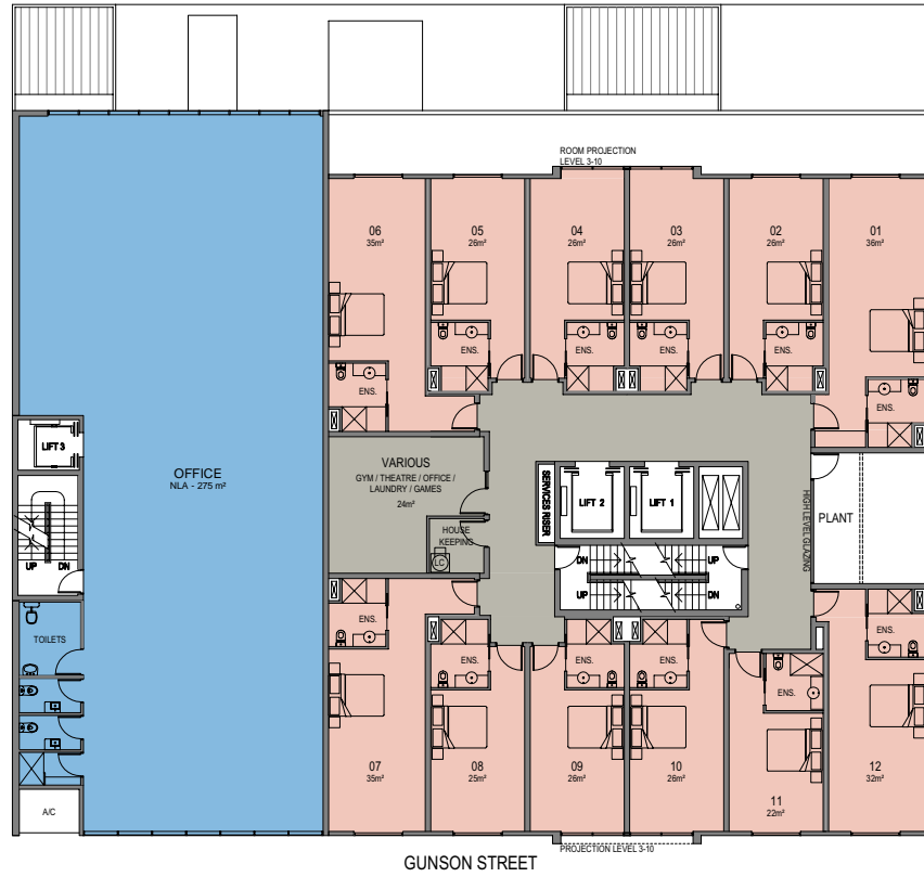
TYPICAL HOTEL & OFFICE FLOOR PLAN (LEVEL 2 - 7) SCALE 1:100 @ A1
