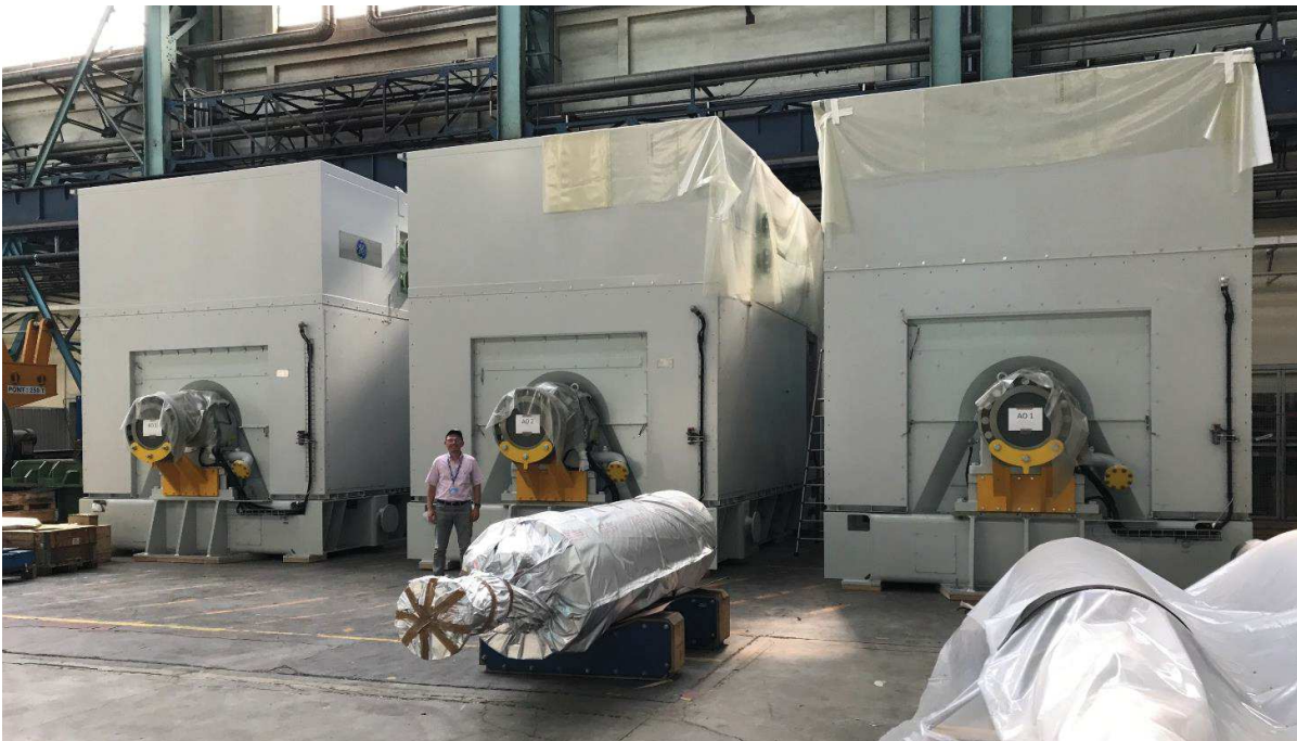
Figure 4-6 Example Synchronous Condensers
