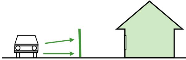
*The barrier must be high enough to block line-of-sight between the noise source and the point where noise may enter your house*
