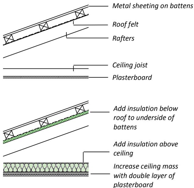
The additional layer of plasterboard can normally be direct fixed to the existing ceiling, increasing the mass and thickness of the system and improving the noise reduction.
