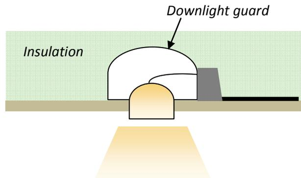
Downlights can pose a fire hazard when covered with insulation. Suitable clearance should be provided or downlight guards installed.
