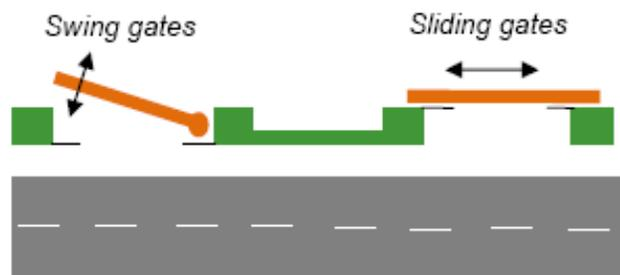
*Overlap sliding gates at the ends where possible, and provide plates at the ends of swing gates to cover gaps.*
