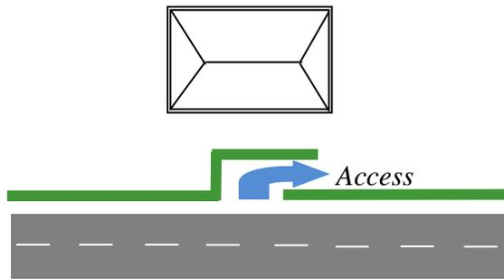
Overlapping barrier sections can be used to provide access without compromising acoustic protection. However it is important to consider the principles of Crime Prevention through Urban Design, ie minimising potential hiding spots for offenders (particularly adjacent footpaths).
