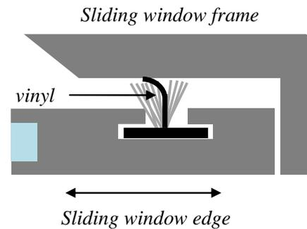
Typical operation of a vinyl fin seal for sliding windows and sliding, glazed doors. It is important that the vinyl fin contacts the window frame.
