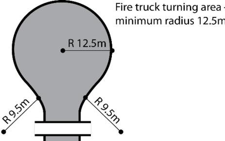
**Figure 5 - 'T' or 'Y' Shaped Turning Head**
