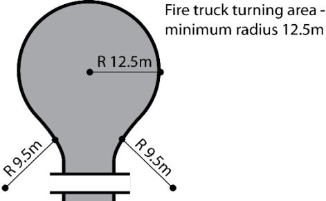
Figure 5 - 'T' or 'Y' Shaped Turning Head
