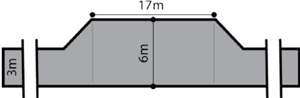
Passing bay for fire trucks - minimum width 6 metres, minimum length 17 metres.
