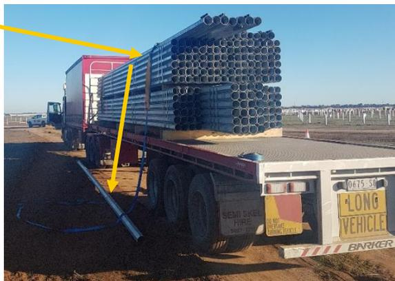
Single top layer of torque tubes secured only by ratchet straps
