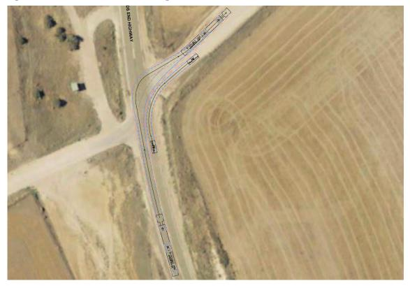
Figure 4.4: 26 Metre B-Double Turn Path - Right Turn into Powerline Road
