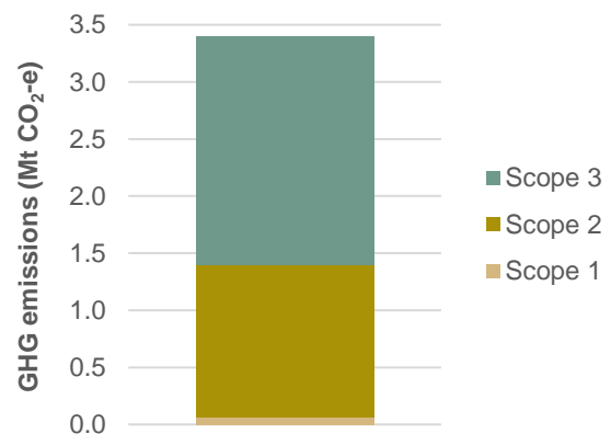
Figure 2 | Breakdown of Scope 1, 2 and 3 emissions for a current practice tunnel project (SA grid)
