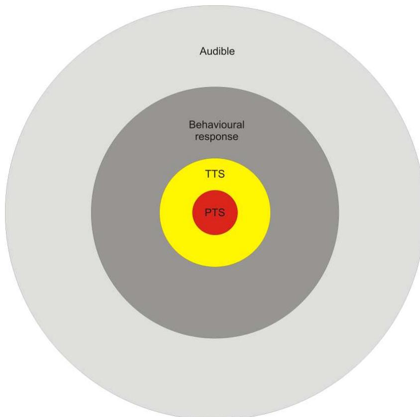
**Figure 5 – Impact zones for underwater noise sources, including zone of audibility, responsiveness, and hearing injury. The zone of hearing injury is further divided into temporary and permanent threshold shift (TTS and PTS) zones.**
