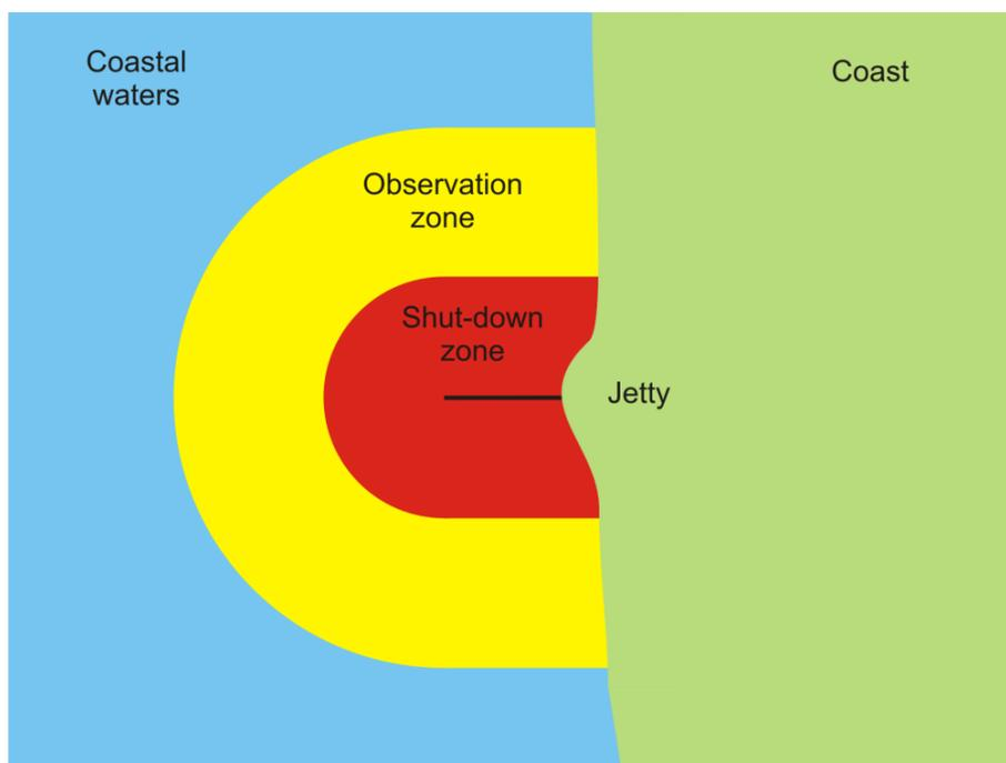
Figure 6 – Diagram showing safety zones around a jetty.
