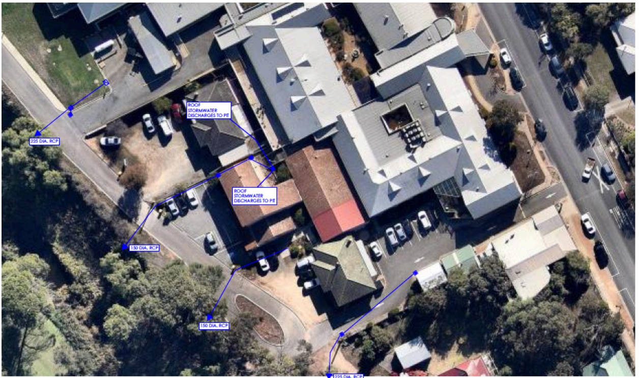
Figure 4 Site stormwater plan, Alfred Place and Angus River discharge.
