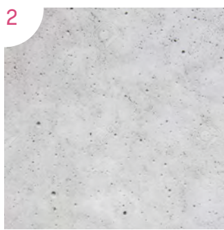
PRECAST CONCRETE. LIGHT GREY OXIDE MIX, SANDBLASTED FINISH
