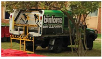
Figure 4-3 On-site bin wash system for rear-lift trucks on back of ute. Source: http://binforce.com.au/
