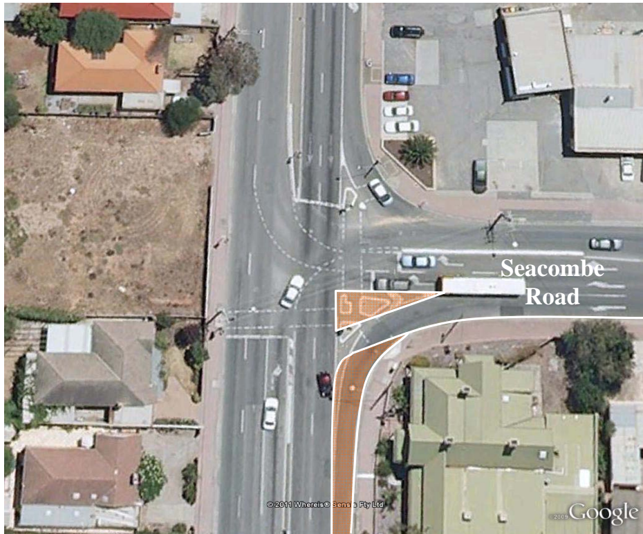
Figure 6-6: Proposed Brighton Road / Seacombe Road Improvements
