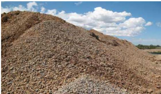
Figure 4: Reclaimed Rail Ballast
