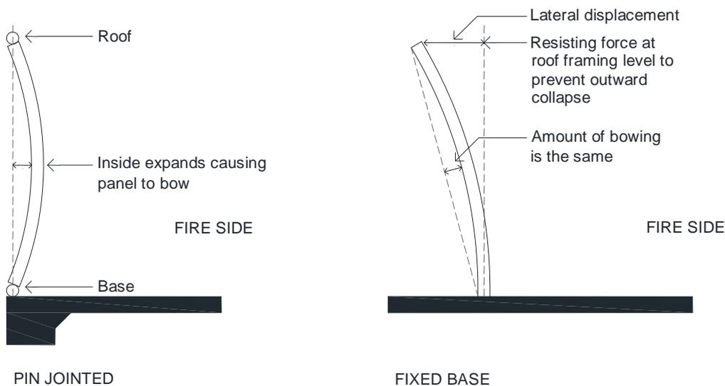
**Figure 3(b) Behaviour of concrete panels exposed to fire**
