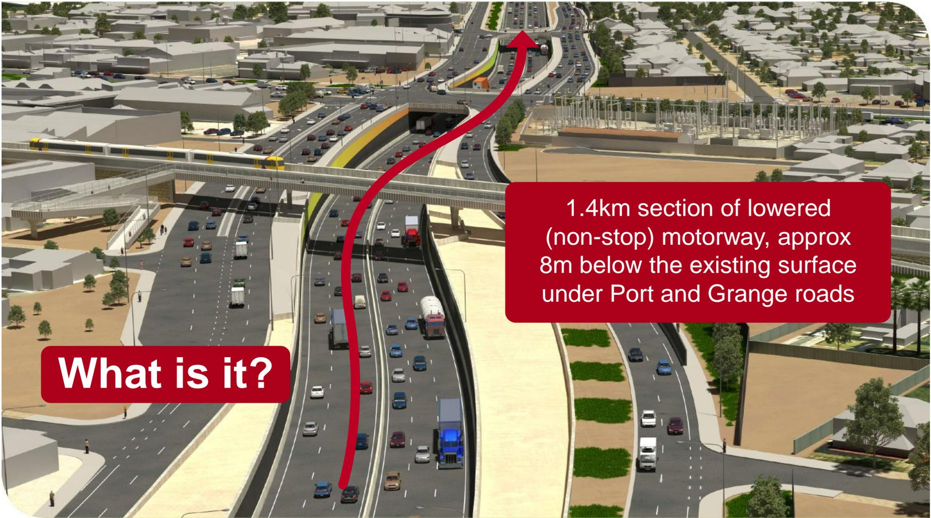
1.4km section of lowered (non-stop) motorway, approx 8m below the existing surface under Port and Grange roads
