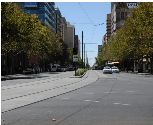
Locating the rail corridor in the middle of an existing road corridor can lessen the overall noise impact.
