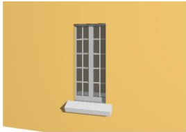
casement window with dressed stone sill
